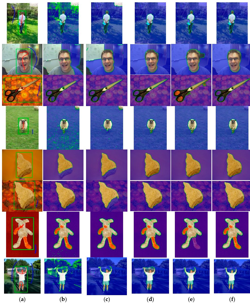
Figure 12. Segmentation results on the GrabCut image dataset for different algorithms. (a) Interaction markers; (b) GraphCut; (c) Lazy Snapping; (d) GrabCut; (e) MSRM; (f) proposed algorithm.
